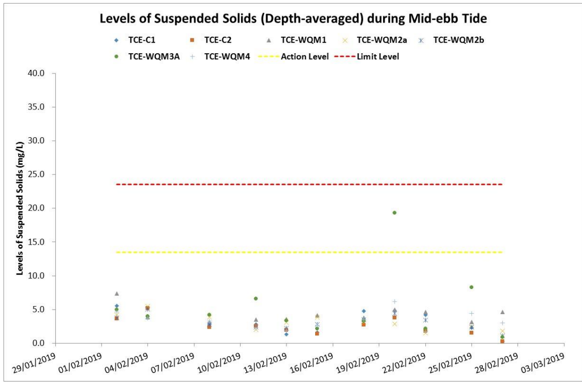
Figure 7: Levels of Suspended Solids (Depth-averaged) (mg/L) recorded at Mid-ebb Tide during the Water Quality Monitoring between 1 and 28 February 2019
